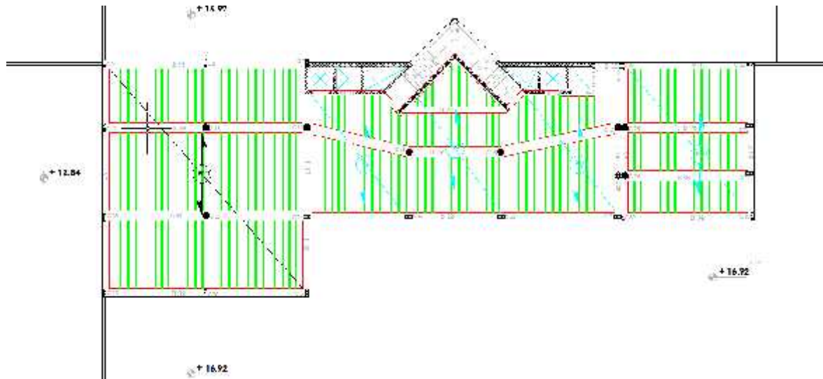
Fig. (4 - 3) Rib location in 4 th floor slab.
