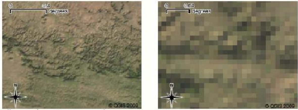
Figure(2-6) Raster data by satellite, the same area to the left with zoom in.
