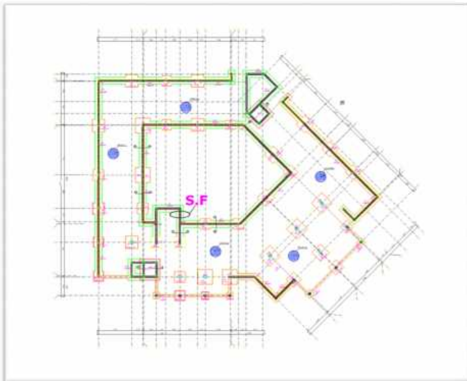
Fig. (4-17). Strip Footing location
