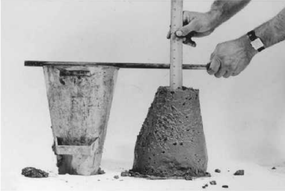
Figure 3.5 Demonstration on use of a slump cone: (top) a low slump and (bottom) a high slump. (From the Canadian Portland Cement Association. With permission.)
