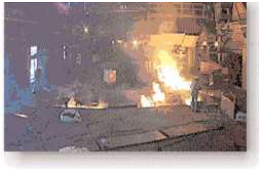
figure3.1: molten slag is diverted to a granulator.
