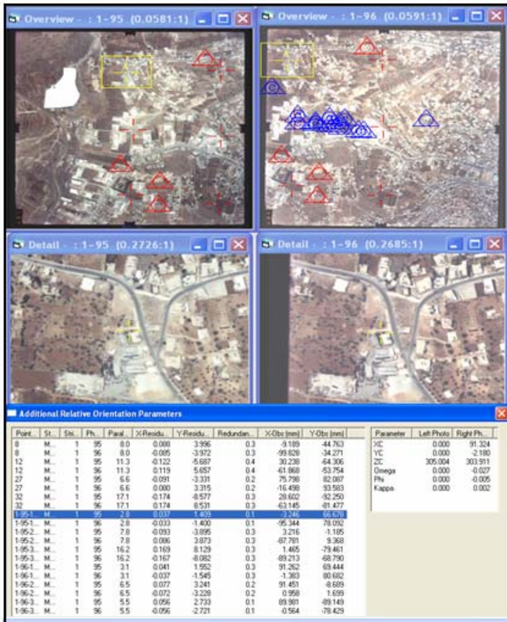
Figure (5-5): Relative Orientation solution for the industry area model using scan resolution 50µm and grid size 10m.
