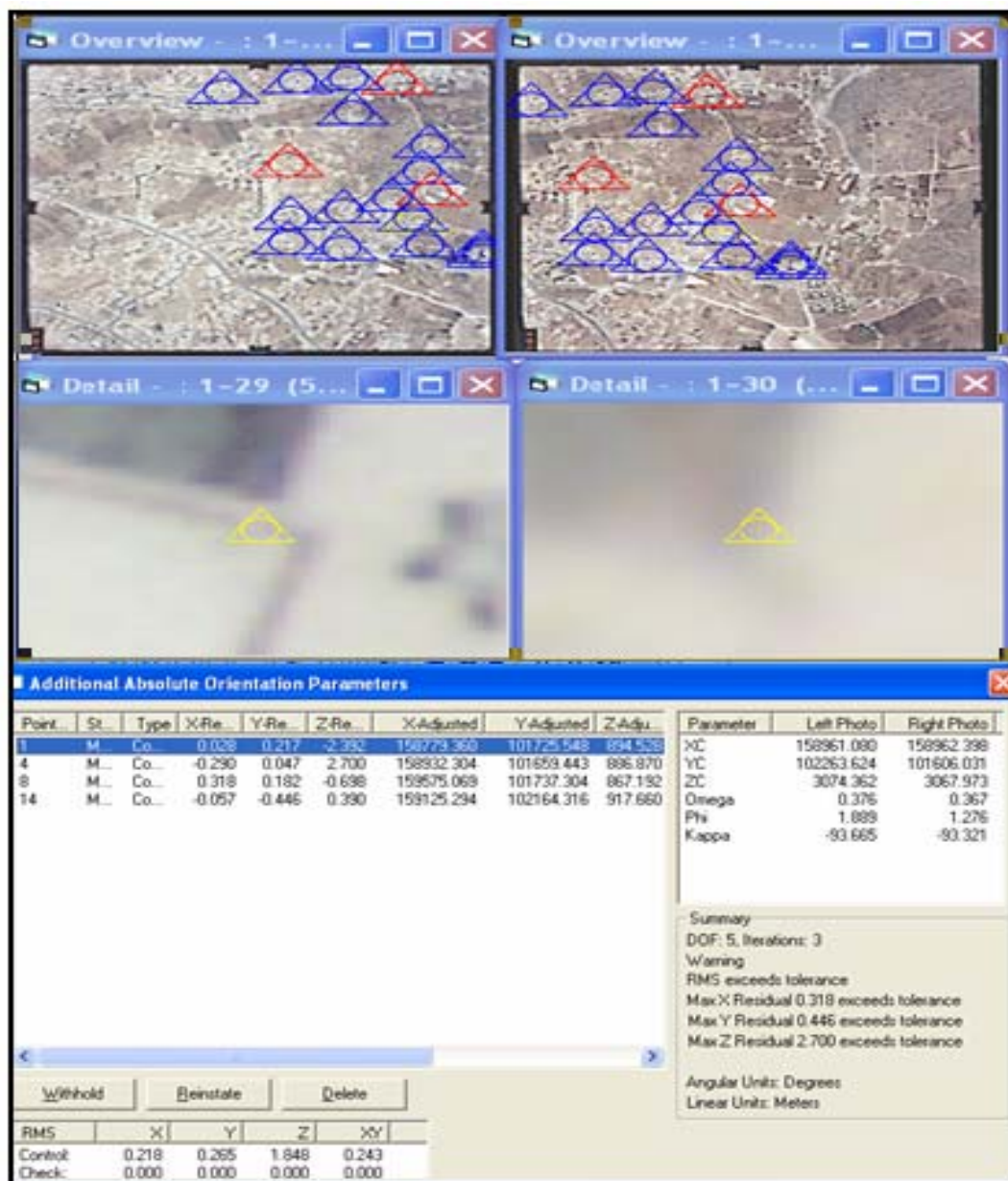
Figure (5-13): Absolute orientation solution for the Wadi Al Harriah area model using scan resolution 20 \mu m and g size 5m.
