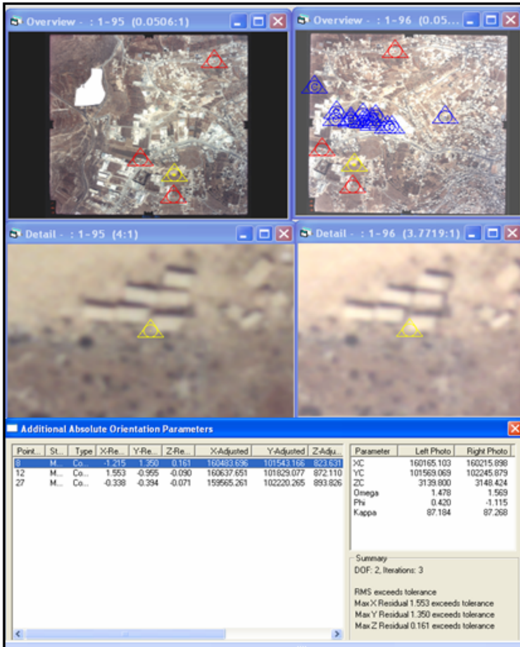
Figure (5-6) : Absolute orientation solution for the industry area model using scan resolution 50µm and grid size 10m.
