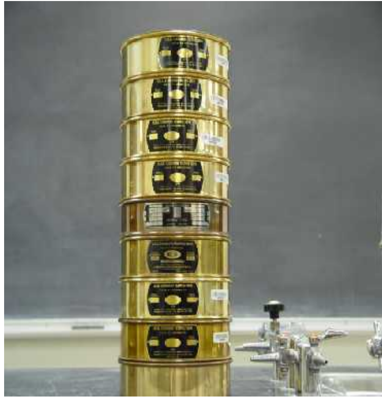
Figure (2.3): Arrangement of Sieves Set (Reference 12).
