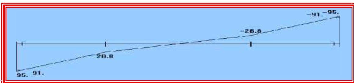
Fig. (4.20): Shear diagram of stairs.
