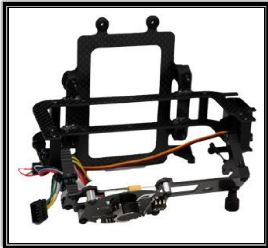
Figure (2 - 4) Aerial camera, with electronic and aircraft mountings. [12]
