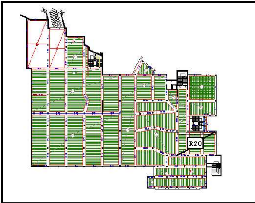
Fig.(4-6) Rib location
