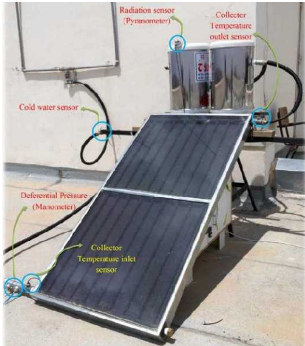
Figure(2.1): Experimental solar system with sensors locations.
