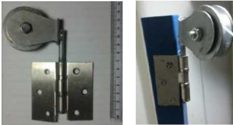
Fig (3.9)Cable pulley
