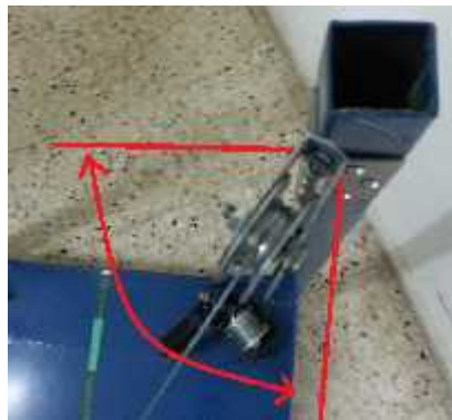
Fig (3.10)motion of pulley cable
