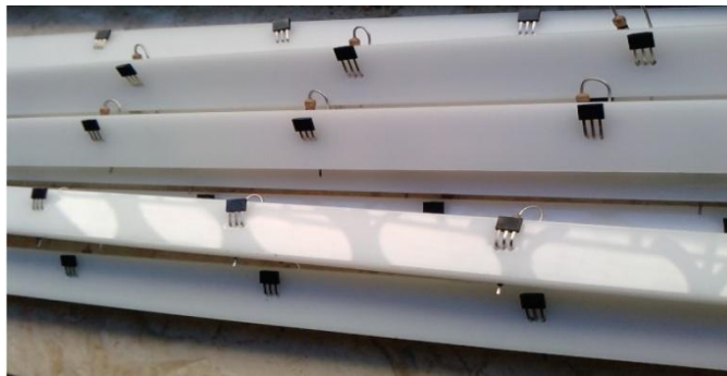
Figure (5.3-B): Magnetic sensors fixed on bars.
