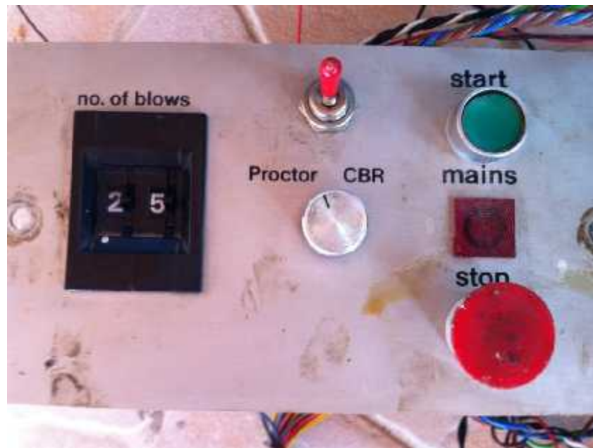
Fig (3.9): Control panel
