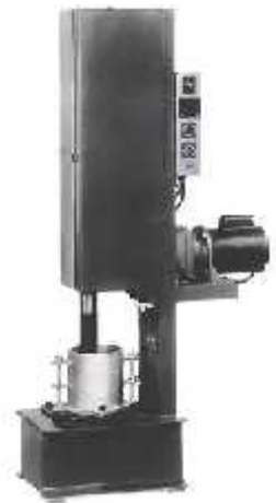
Fig (1.1): Compaction Machine
