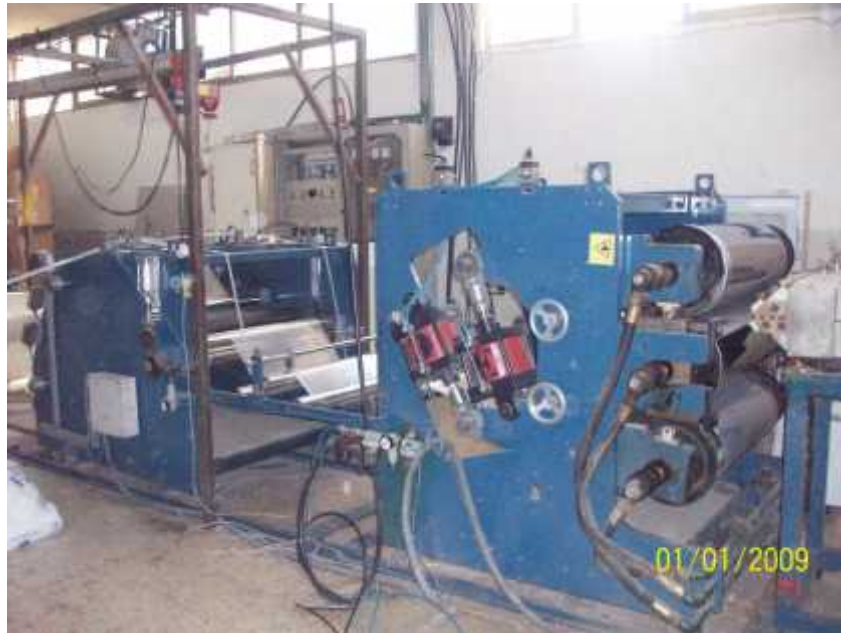
Figure 2.3: The second section of extruder machine
