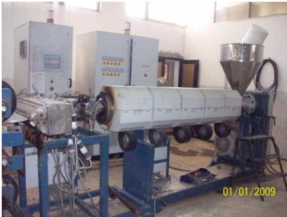
Figure 2.2: The first section of extruder machine
