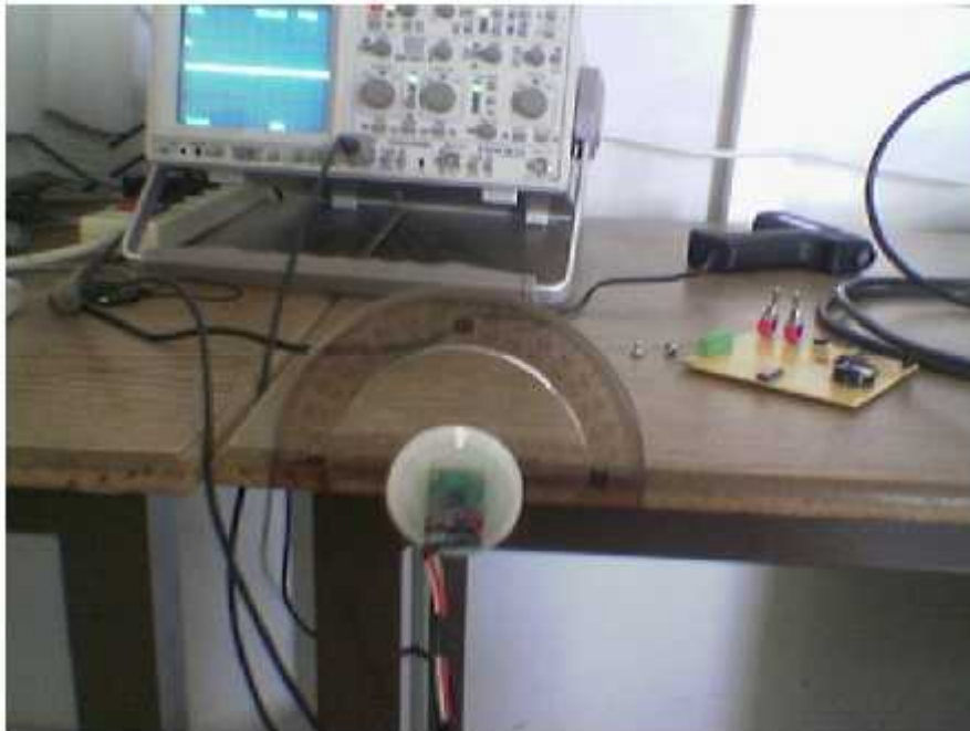
Figure5.5 Calculating the sensitivity gain for the accelerometer in the Lab.
