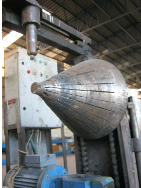
Figure 2.6: Shows the knife holder in cutting position.
