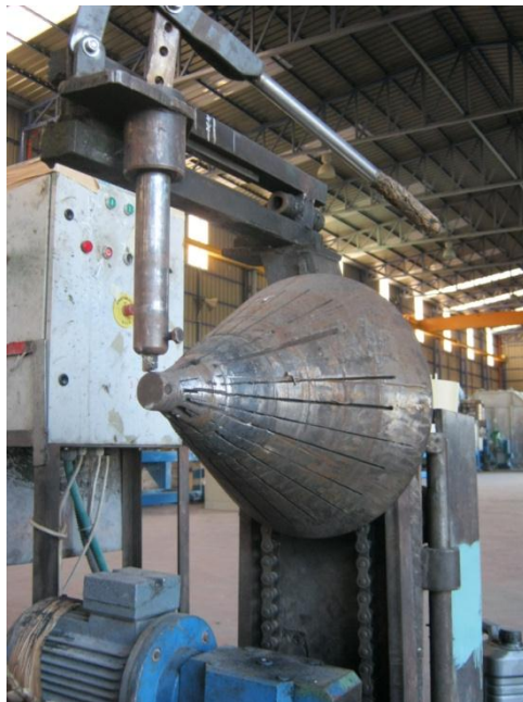
Figure 2.5: Shows the knife holder in normal position.
