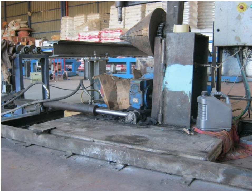
Figure 2.1: The end of the slider, and how there is no limiting boundary that stop pipes from falling.
