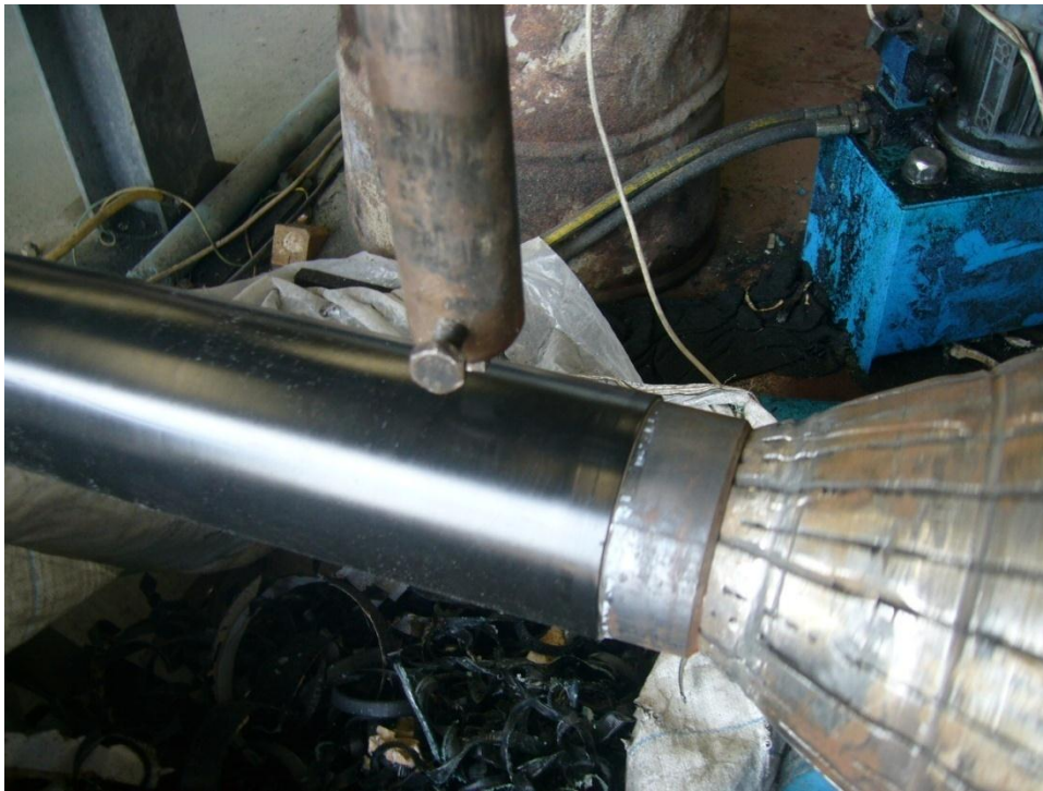
Figure 2.2: Pipe fixing and rotating through cutting operation.
