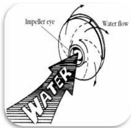
Figure (6.6) : Working method of centrifugal pump.
