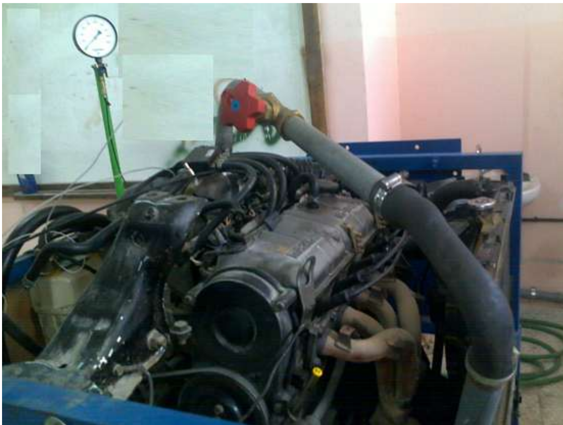
Figure 5.1: Connection pipes between intake and exhaust manifold
