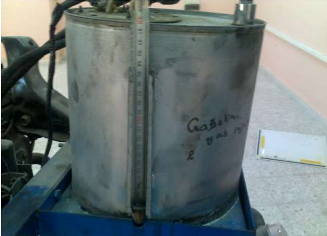
Figure 4.4: Fuel Tanks with Glass Tube Scale
