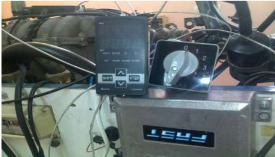
Figure 5.4 device to reading the temperature.
