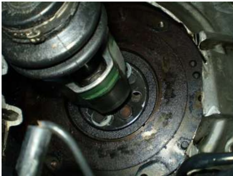
Figure 6.3: The Interchangeable Connection Shaft
