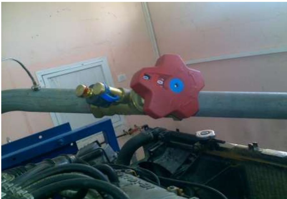
Figure 5.2: EGR manual Control valve
