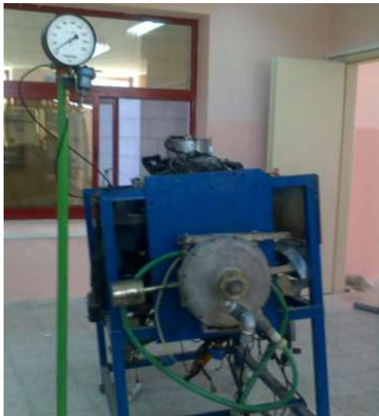
Figure 4.2: Engine Performance Test Stand with Vertical Instrument Panel
