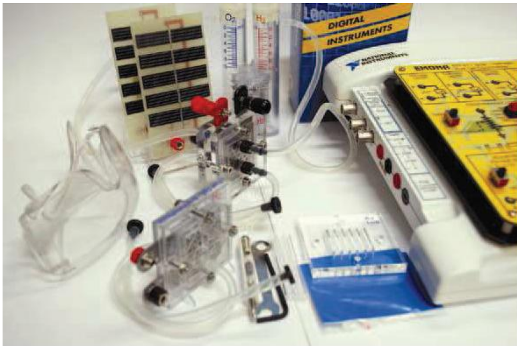
Figure 6.1: The Emona HELEx Add-in Module along with kit components.
