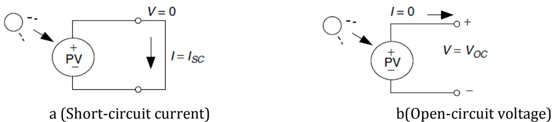
Figure 2.3: Two important parameters for photovoltaic's are the short-circuit current I_{sc} and the open-circuit voltage V_{oc} .
