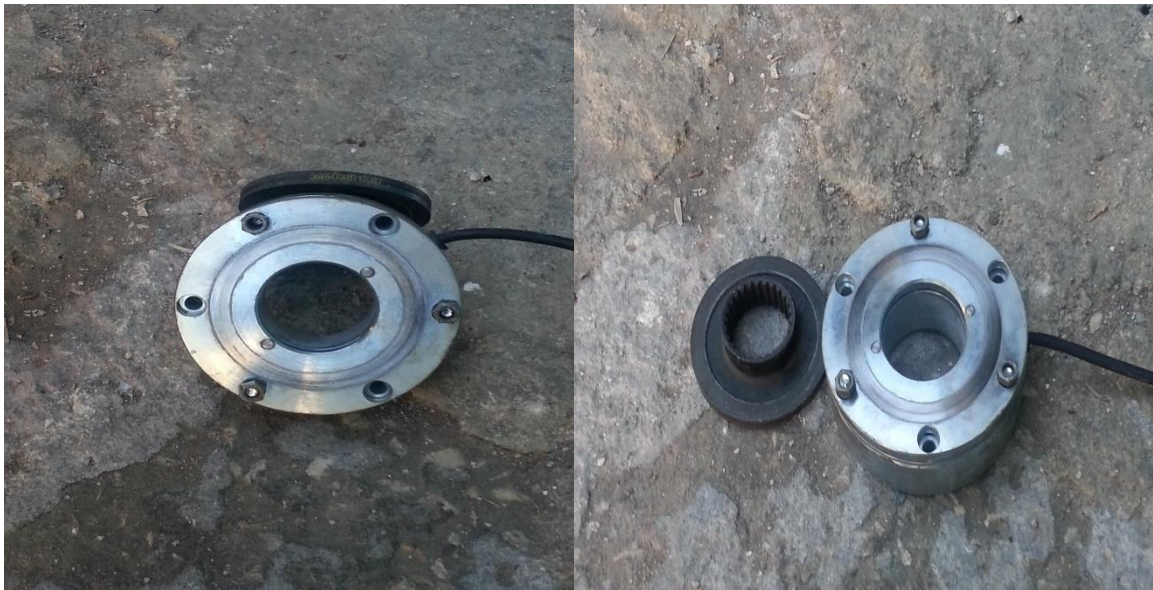
(c) Electric assistant brake connected to the motor as a handbrake (before installation).
