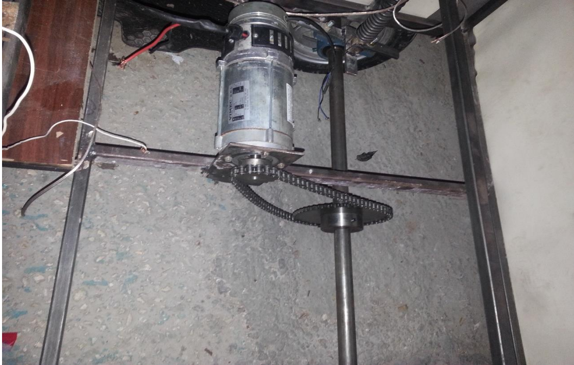
(b) Input and output gears with chain after connected to the motor.
