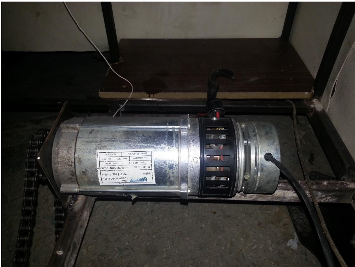
Figure 3.1: DC motor installed in the vehicle.
