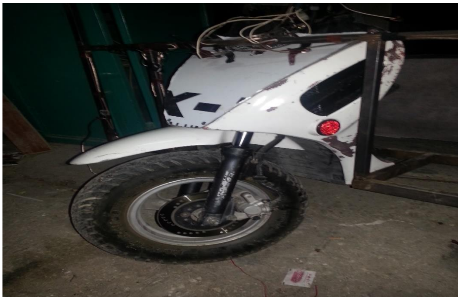
(b) Front view of front tire after installation.
