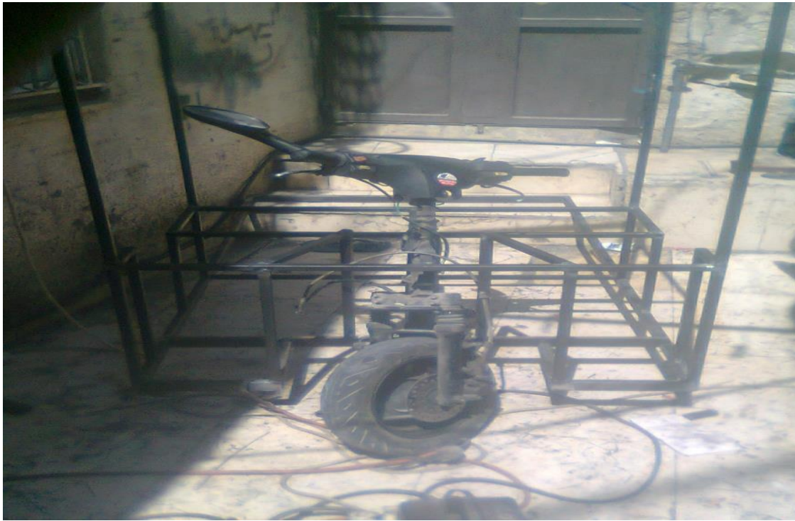
(c) General shape of chassis with steering system installed.
