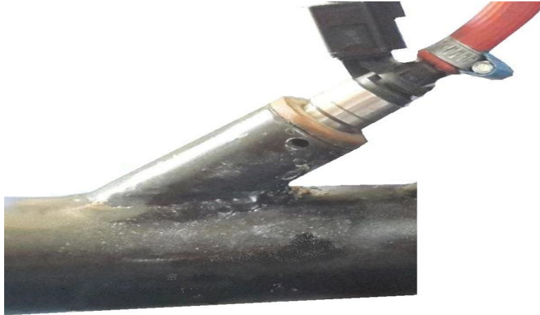
Figure (3.21): Injector isolation using wood fiber.
