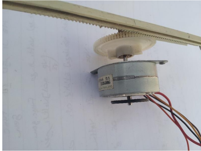
Figure 4.9 Stepper motor with rack and pinion.
