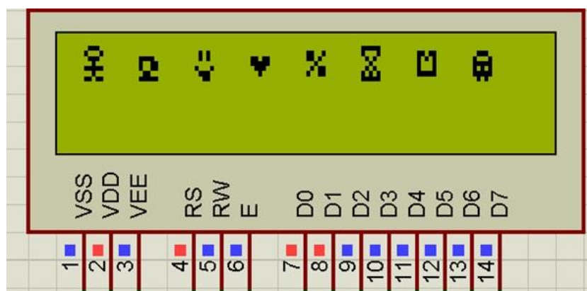
Figure 3.10 LCD Pins And Simulation Of Special Character.
