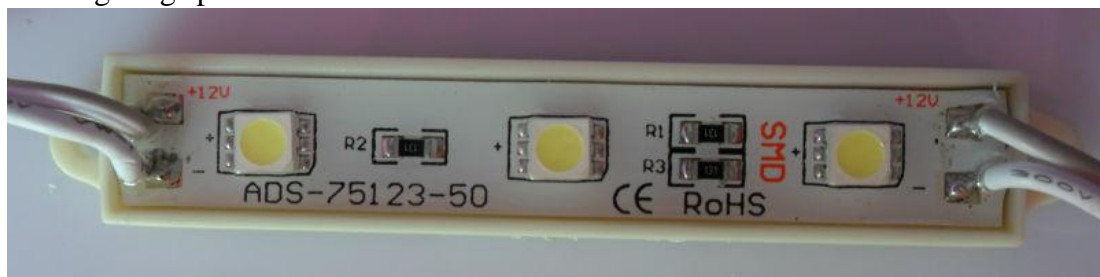
Figure 3.19 LED Lighting used in CUC 0.72 watt
