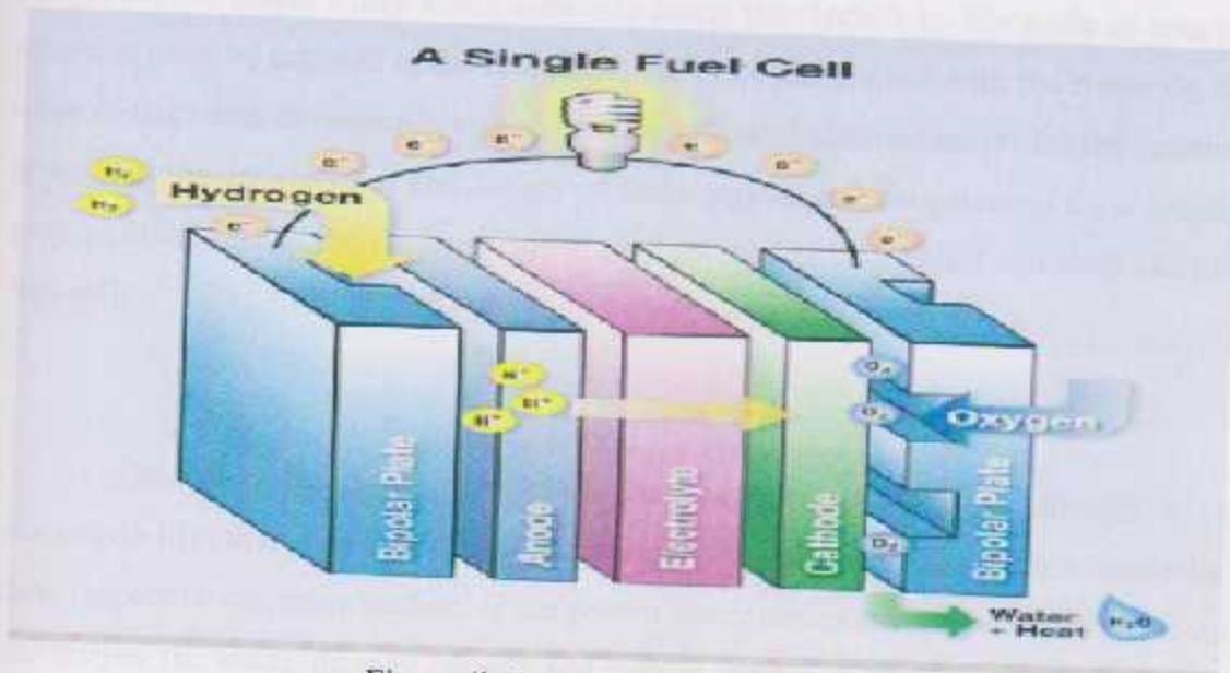
Figure (2.1): Fuel cell Basic Structure
