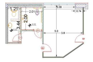
Figure 2.3: Dimension of back office and W.C:
