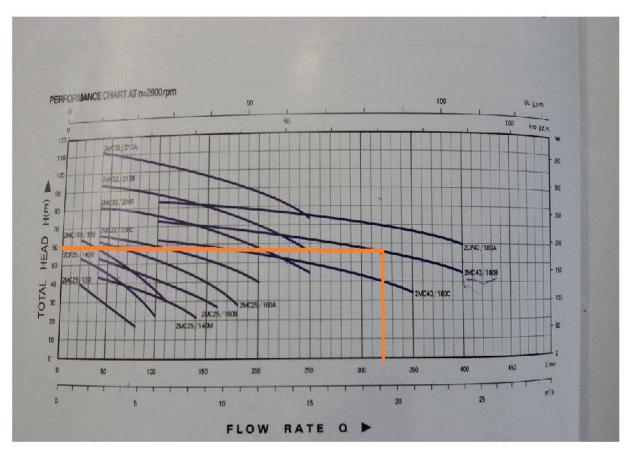
Figure 5.13: Pump characteristic curve
