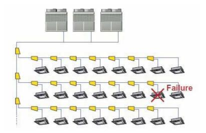
Figure 3.6 : Continuous operation is possible even if trouble occurs at an indoor unit.[6]
