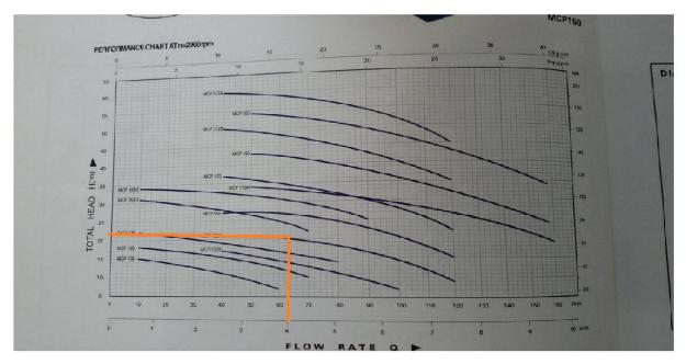
Figure 4.4: Pump characteristic curve
