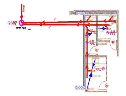
Figure 4.6: Distribution of piping in bathroom
