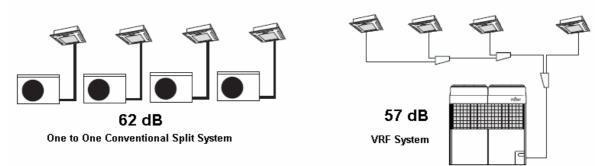
Figure 3.5 : One to one conventional split system (62dB, 57dB)
