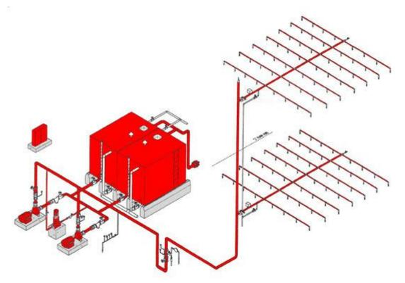
Figure 5.7: Automatic sprinkler system
