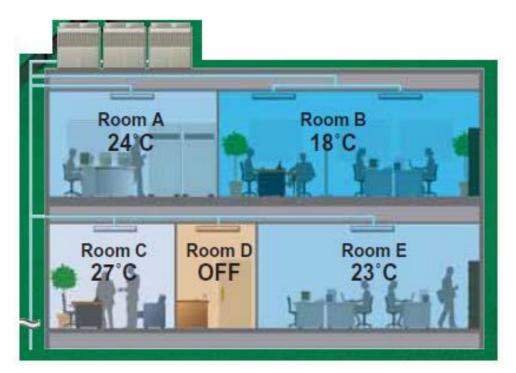
Figure 3.4 : Advantage of a variable refrigerant flow system
