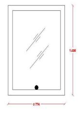
Figure (2.5): Dimensions of window
