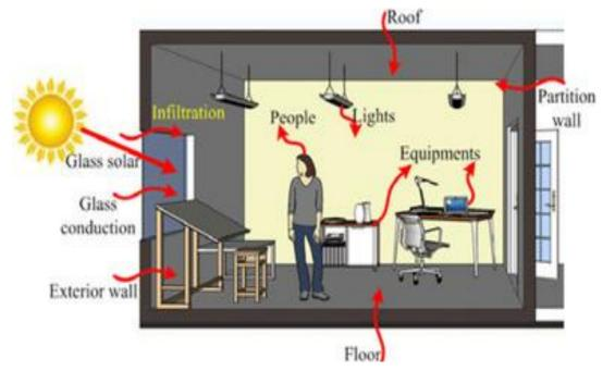
Figure 2.6: Source of cooling load [4]
