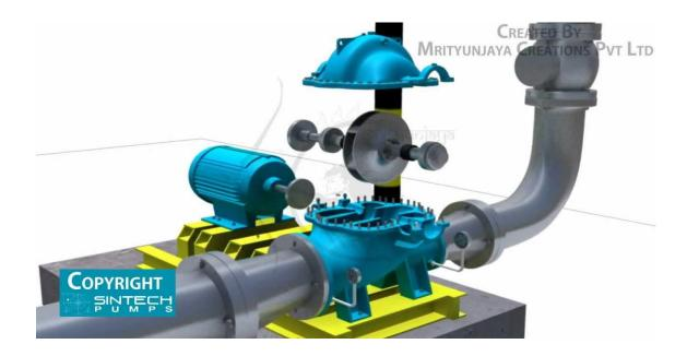
Figure 5.9: Horizontal split case pump
