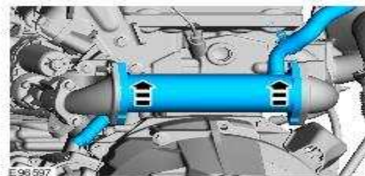
Figure 3.7:Connected EGR cooler.
