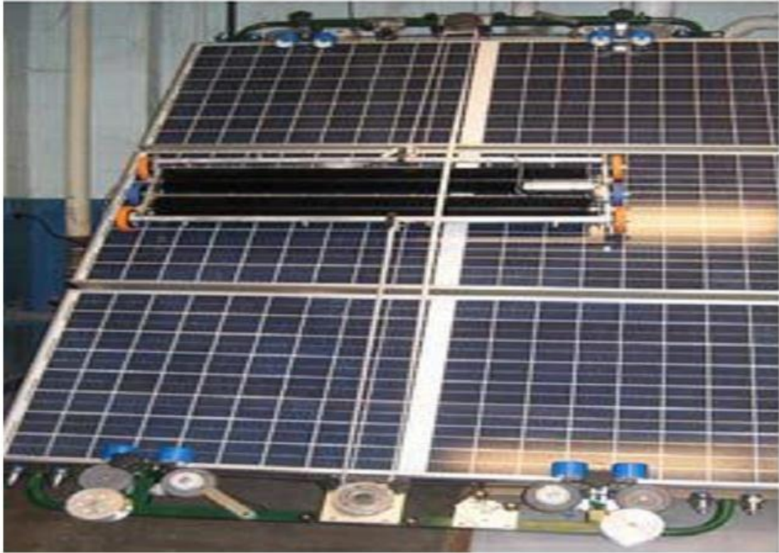
Figure 2-4: Traveling system of robot V1.0 head along of the panel arrays
