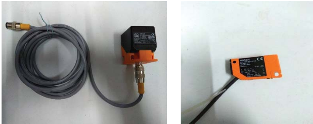
Figure 7.7: Magnetic and Inductive sensor
