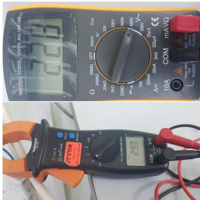
Figure4.12: Load voltage and current of PV and battery
