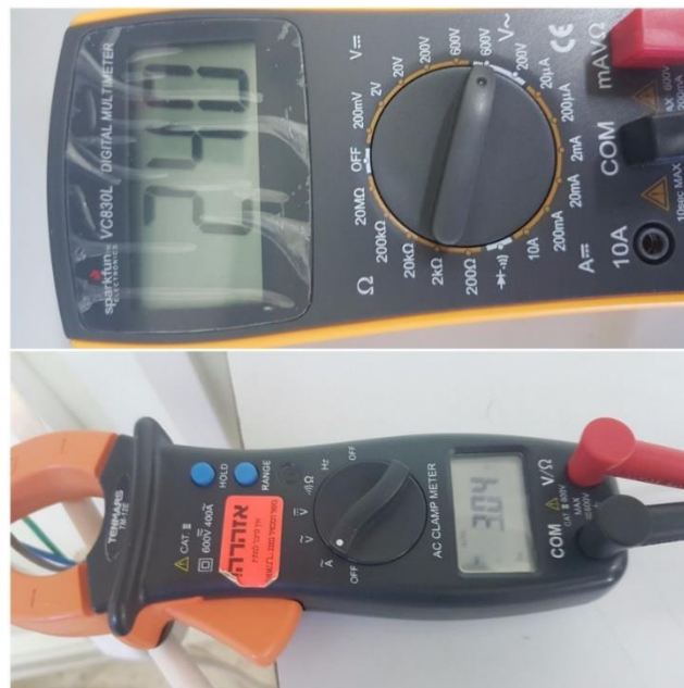
Figure 4.10: Load voltage and current at grid connected.
