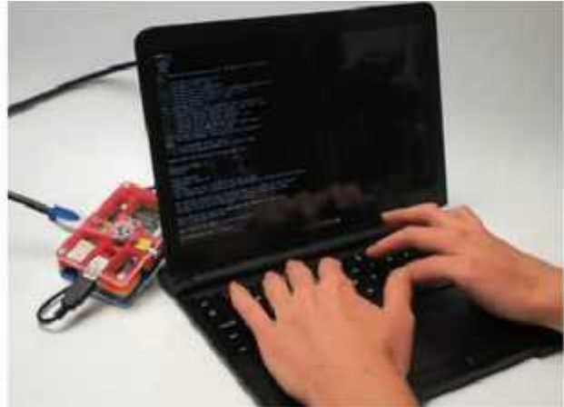
Figure 4.1 Installing Raspbian operating system 1
