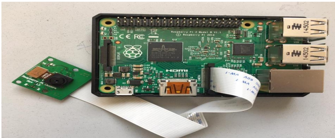
Figure 4.2: Connecting raspberry pi camera to the Raspberry pi
