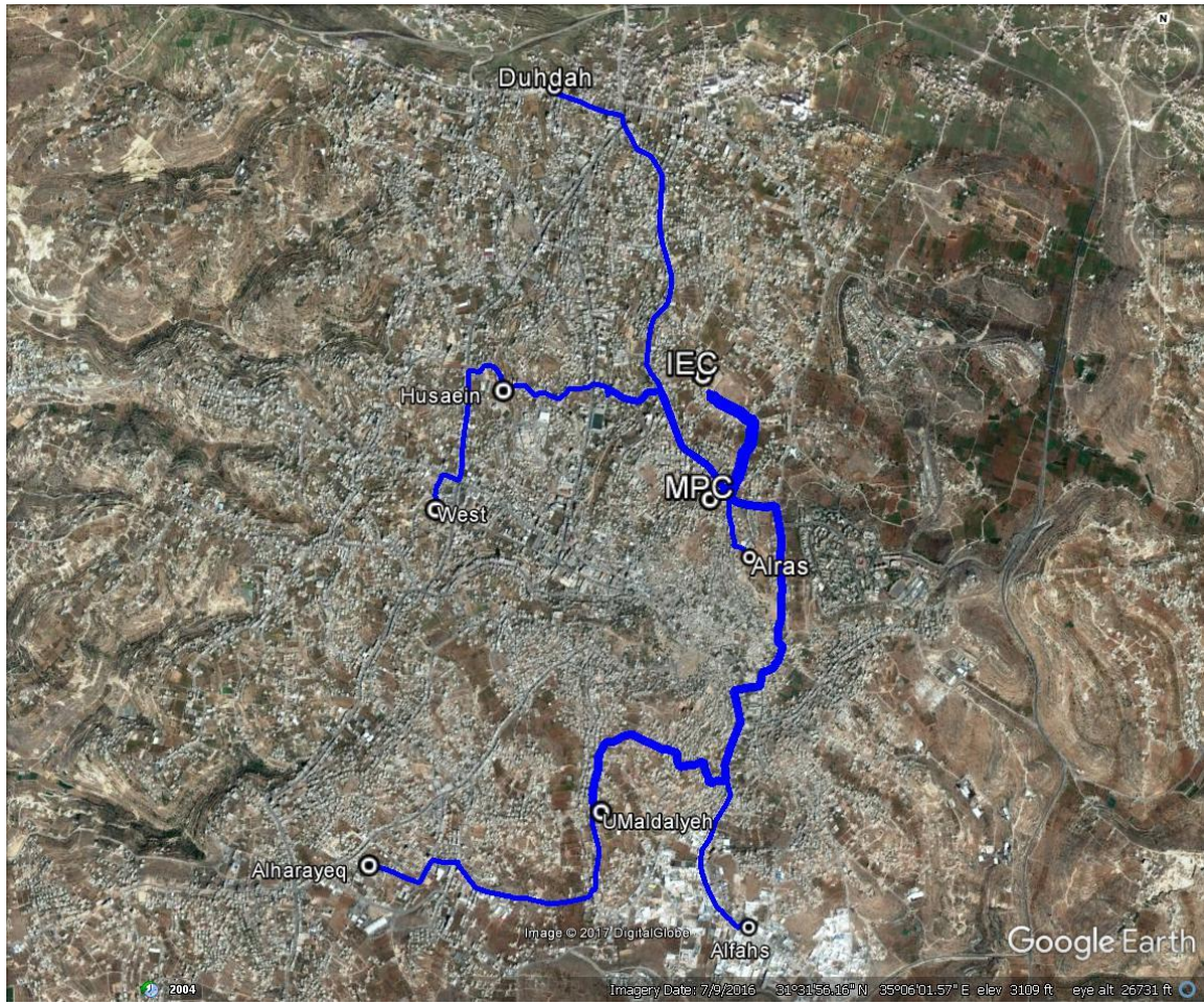
Figure (4.4):33kV Network
