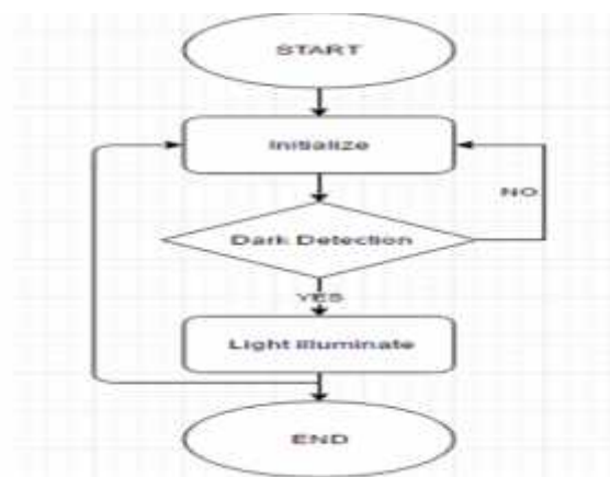
Figure 4.4: Flow chart of LED indicator
