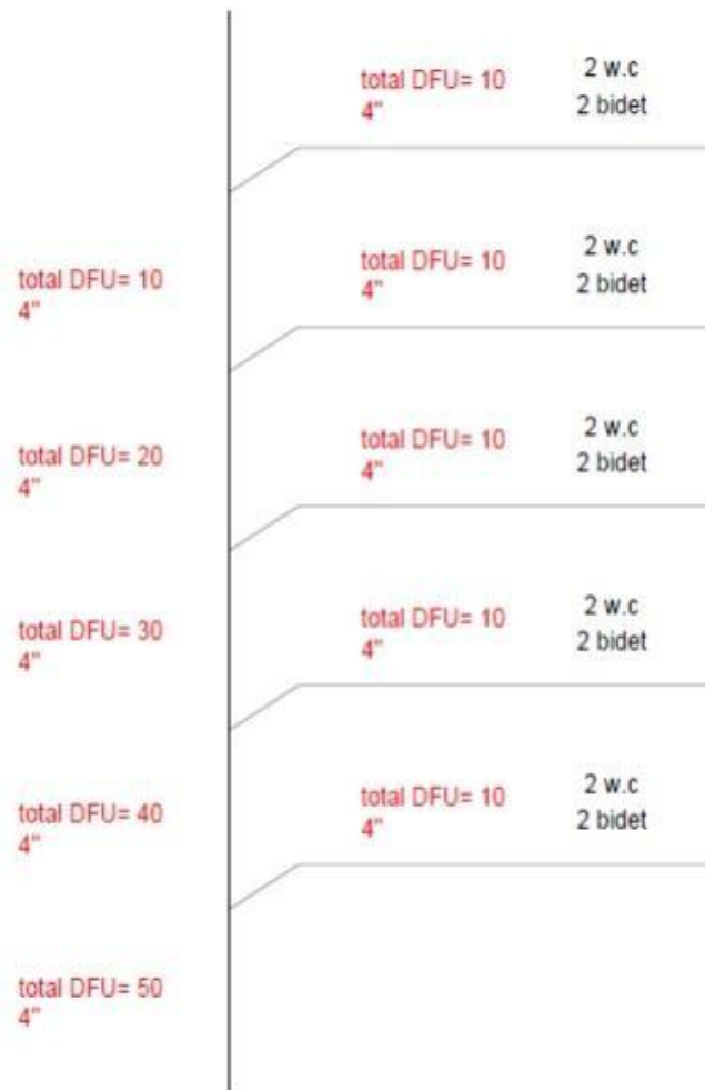
Figure 4.9: Sample of black water stack 1
