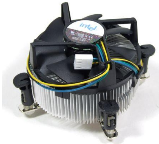
Figure 2.4: Heat Sink Design.
