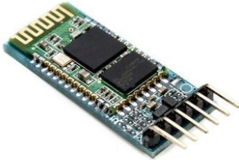
Figure (2.6): Bluetooth module (HC05).
