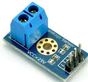
Figure (2.9): Voltage Sensor.
