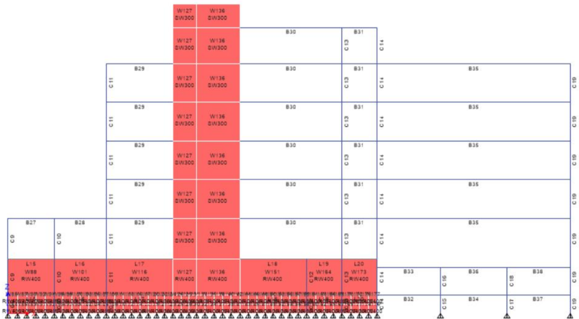
الشكل 35 Shear wall at axis 3
