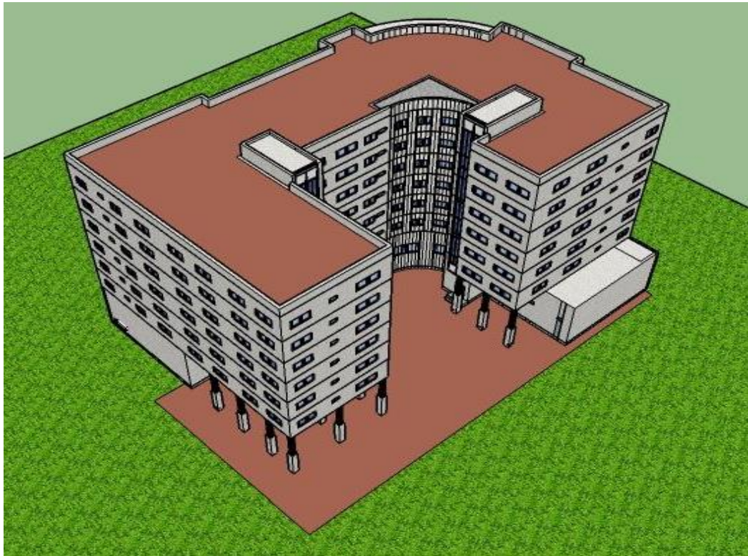
Figure 6.2 The desired area of the building for green roof system in brown colure
