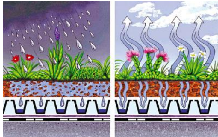
Figure2.4 Provides Rainwater Management[29]
