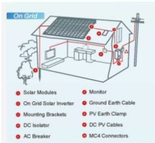
Figure 1.2: On Grid Systems [8].
