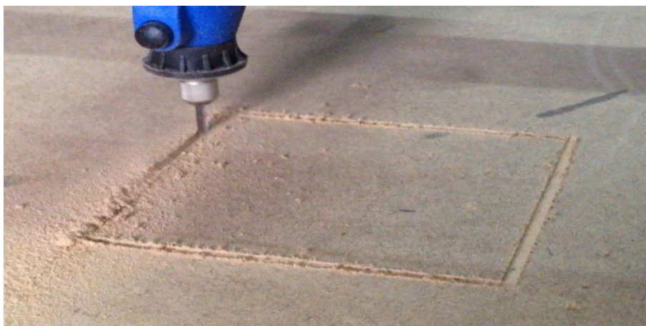
Figure 6.3 Mill Square on Wood.
