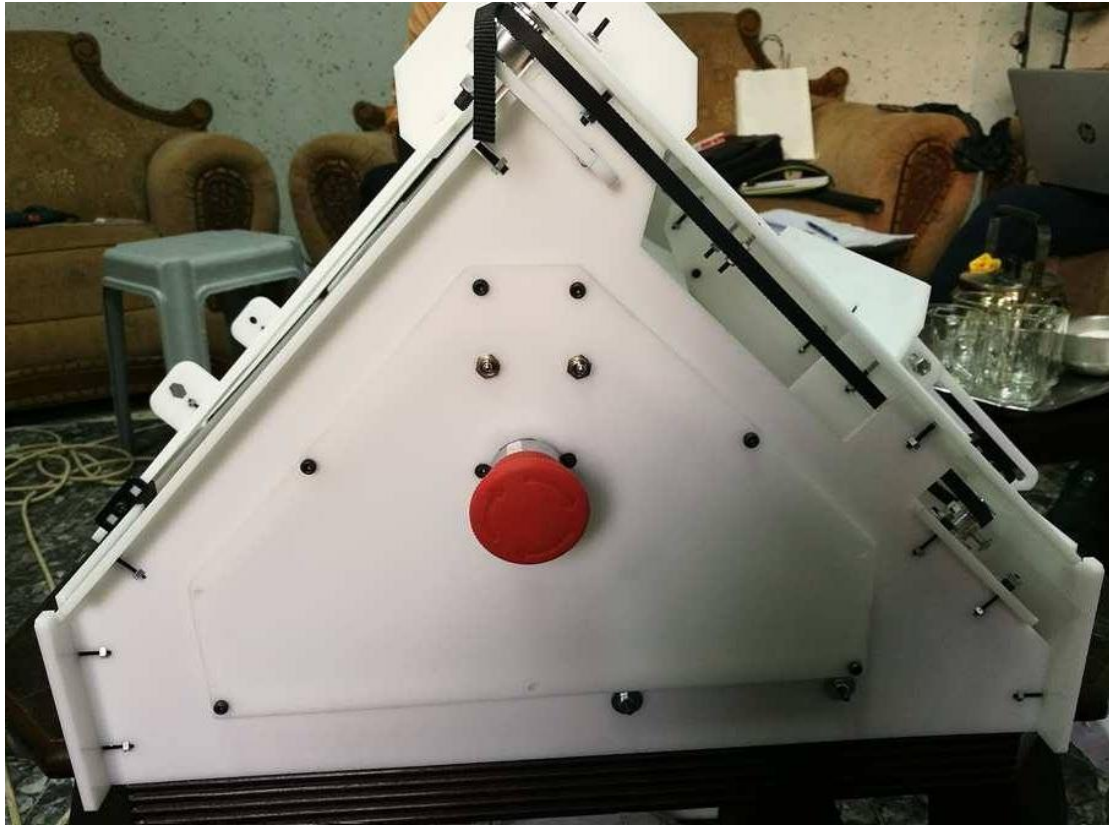
Figure 6.4 Emergency and switches of the system
