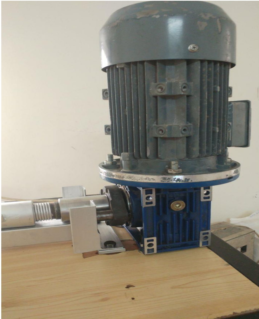
Figure 5.8: auger was attached with a coupler to the shaft of the motor.
