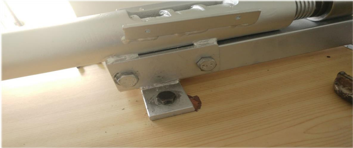
Figure 5.6: extruder structure installed with frame.
