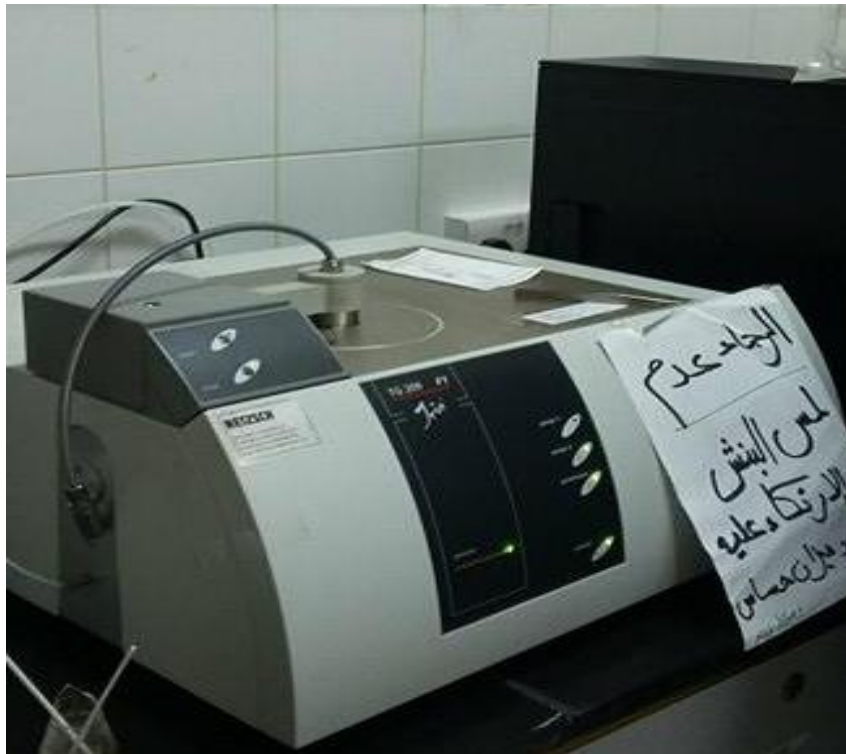
Figure (4.7): Thermogravimetric analysis (TGA) test device.
