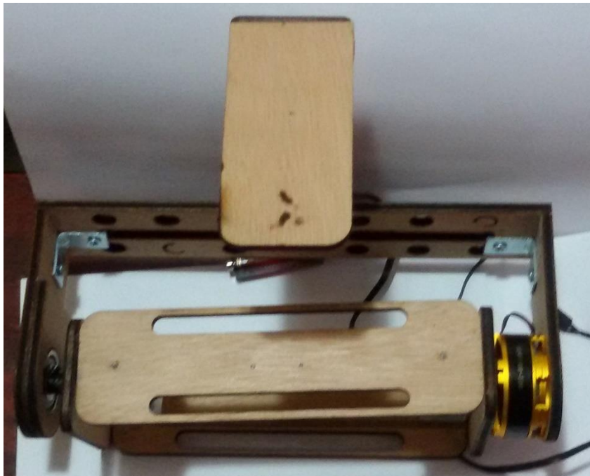
Figure 5.13: The Stabilizer After it had been Assembled Practically
