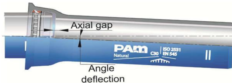
Figure 5. 4: Standard Vi Joint for pipes
