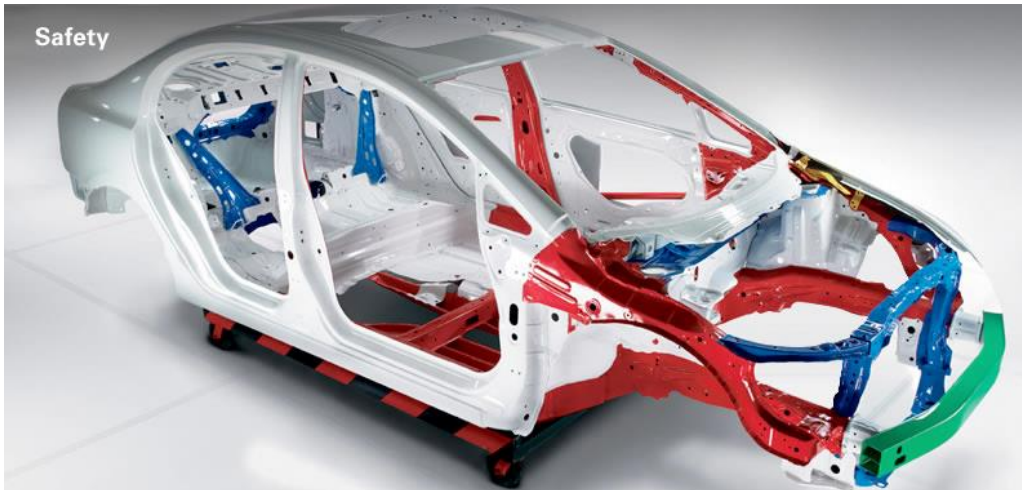
figure (9): unibody frame
