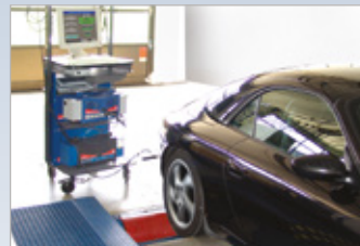
Connection to LPS function and performance dynamometer
