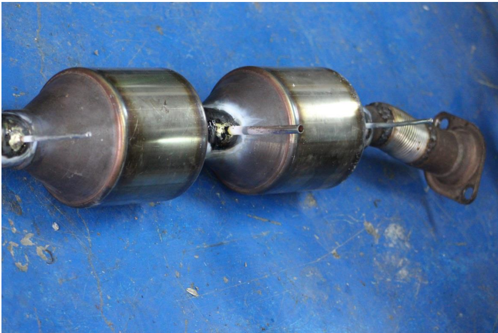
Figure 4.6: Double catalytic converter layout
