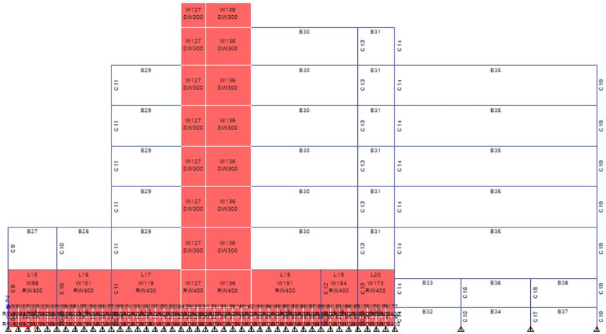
الشكل 35 Shear wall at axis 3
