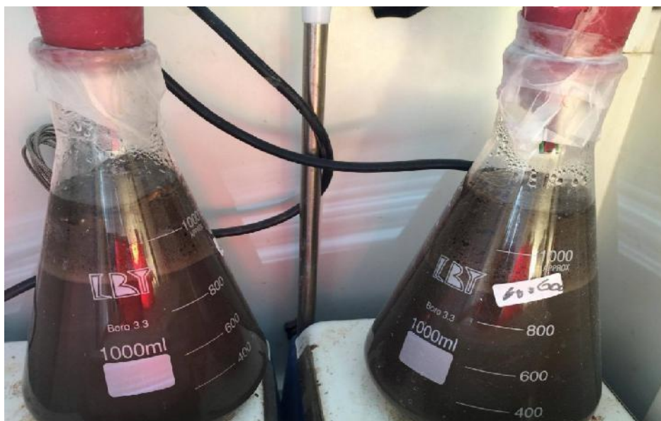
Figure 4.1 : The appearance of scum layer in the ABR.
