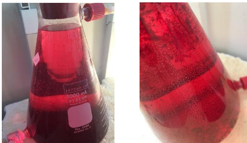
Figure 4.2 : Bubbles in the gas collection system.
