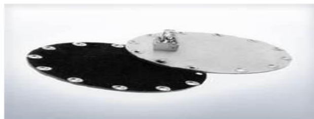
Figure 3.6: Microstrip antenna used in radar.
