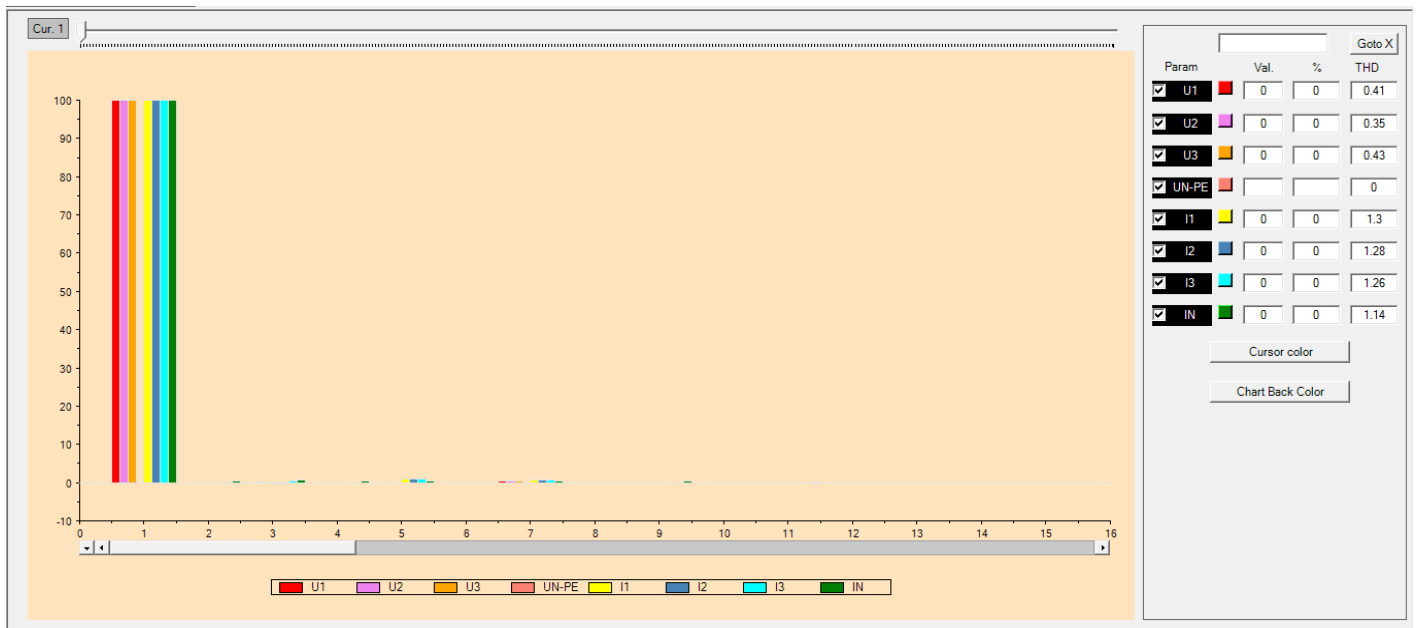
Figure 3. 5: Harmonic in current and voltage of KHALAT LOZA Transformer.
